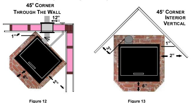
Note: If interior vertical vent is used, the clearance to the back wall is determined by the upward-turned elbow or "Tee". It will vary in depth depending on the brand of PL vent used.
